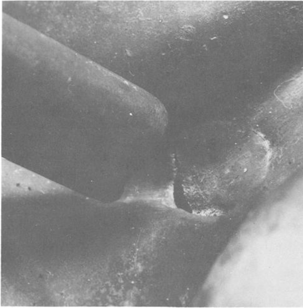
FIG. 3—This close-up photograph of Position 2 on the gas tank shows that the hole can be matched with the top, sharp edge of the stand.
